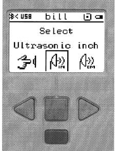
ultrasonic sensor is usually uses Port 4.
