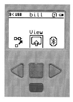
This will open up the view section so you can check the various sensors as well as the rotations of the motors.
