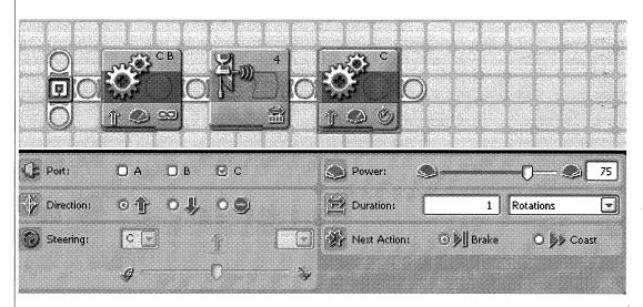
The rotations may need to be changed to make it move back enough that it will not hit when it turns, but close enough to the wall so it does not hit the post on the figure 8.
